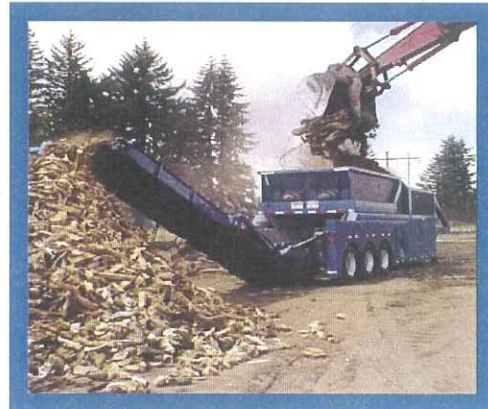
PR-4000 mobile reducer processing stumps
