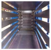
The ram sides feature wear resistant, adjustable, and replaceable Nylatron liners. The floor and ram bottom feature 400 Brinell steel liners. Oversized ram hold-down bars are ajustable and accessible from the exterior of the baler.
