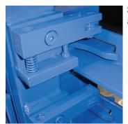
Spring-loaded retainer locks and ajustable wire positioners.
