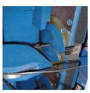
The gear driven (no twister hooks) tier has replaceable wire cutters. The inserter and twisters are driven by hydraulic motors.
