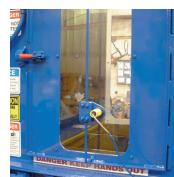
The chute-type in-feed hopper has a gasketed access door and viewing windows on both sides of the hopper. Photoelectric infrared sensors are adjustable the entire height of the door.
