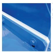
The adjustable and replaceable ram wiper is made of UHMW plastic and is accessible from the exterior of the baler.
