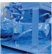
TEFC motor with quiet running 3-section flooded suction pumping system.
