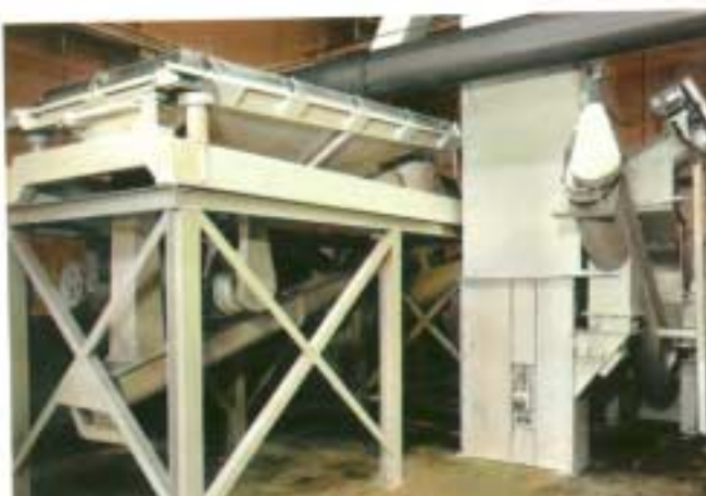
This Model 81 Automatic-Tensioning ROTEX Screener with single split screen is used for screening meat meal. Usable meal passes through at the leading end of the split screen, while oversize recycle material is conveyed toward the discharge end where it passes through the coarser screen mesh section. Hair, fluff and very large oversize material are discharged together off the top.
