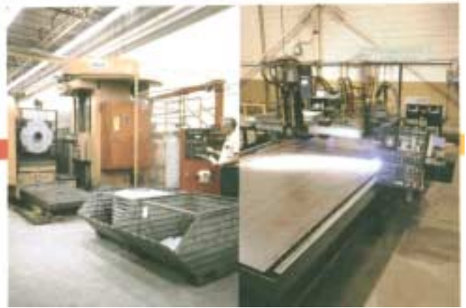
This computer-controlled machining center (left) and computerized cutting table (right) typify the advanced precision methods used in manufacturing ROTEX products.
