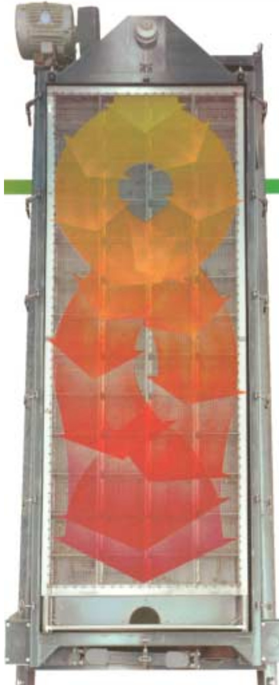
ROTEX Screeners control screen blinding through a system of bouncing balls confined in pockets beneath each screen surface.
