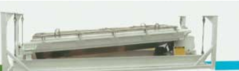
Cable suspension from overhead structure (above_ and from a cradle type floor stand (below)
