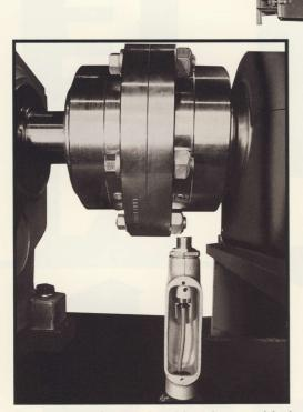
Every top feed shredder is provided with an arbor speed sensor, interfaced with the programmable controller. Each revolution of the arbor is counted automatically. If it slows down for any reason, the infeed conveyor will stop automatically. Under normal conditions, the possibility of stalling out the arbor is eliminated.
