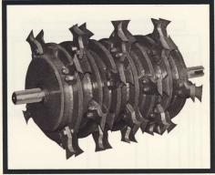
The single arbor design of each top feed shredder features staggered heat treated blades that are bolted to the arbor for easy replacement. Single and double blade configurations are available. Blades are reversible, thereby doubling the life of each blade.
